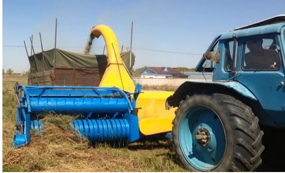
Fig. 5. – Forage pickup chopper PIK-1,8 with new pickup mechanism (Pickup and cutting hay with moisture content 18-20%)
