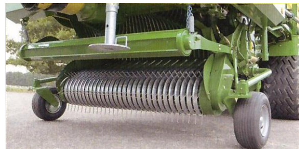
Fig. 2. – Constant pickup device for many models of Krone Easy Flow
