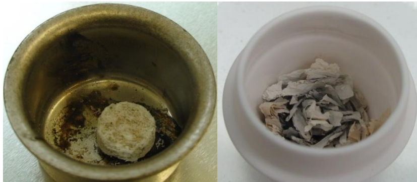
Fig. 3. – a) Ash from incineration briquette, b) the ash from burning of input materials for the production of briquettes
