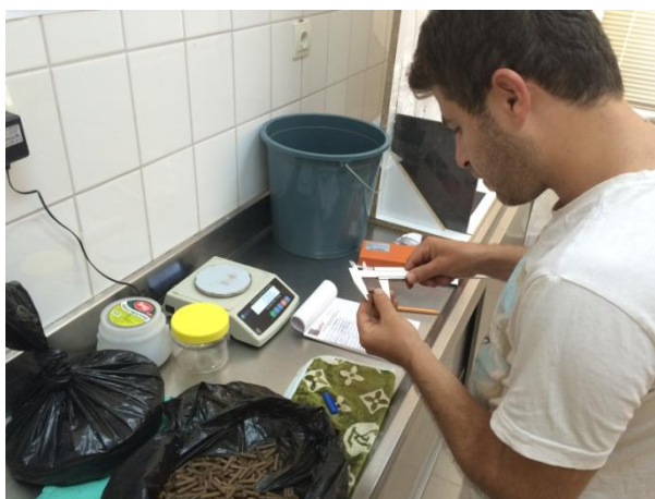
Fig. 5 – Determining some physical properties of pellets
