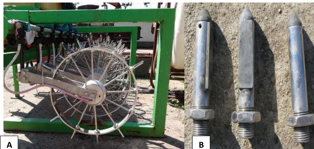
Fig. 2. – Wheels with apices GFI 3A (A) and application apices (B) (A – SEDLÁŘ (2013) and B – KOZLOVSKÝ (2011))
