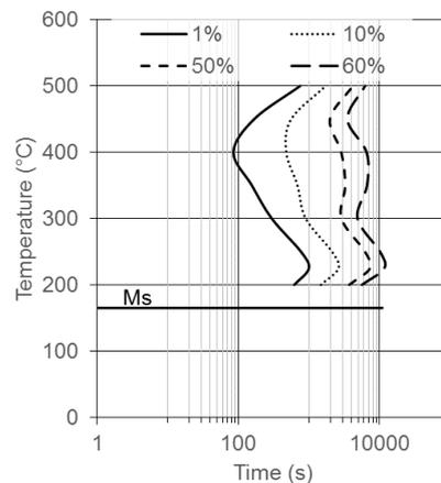
**Fig. 4.** – TTT diagram developed by results from EMS sensor
