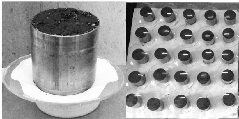
Fig. 2. – Kopecky's stainless steel ring during evaluation
