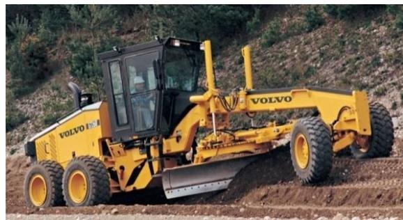
**Fig. 2.** – Ground leveling with grader
