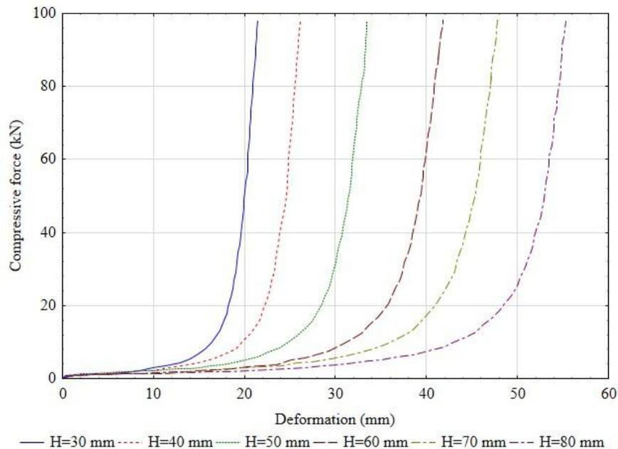
**Fig. 1.** – Dependency between compressive force and deformation curves for different pressing heights of jatropha bulk seeds for vessel diameter 60 mm similar to diameters 80 and 100 mm given by HERAK ET AL. (2013A) AND KABUTEY ET AL. (2013)
