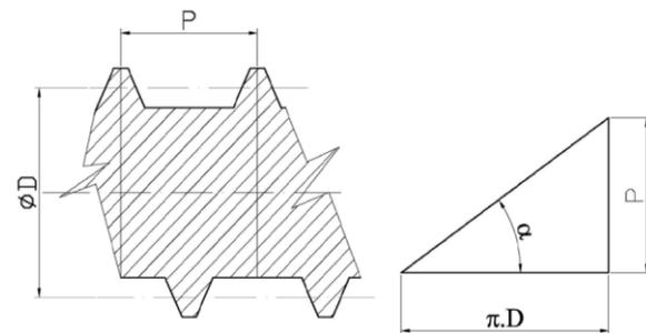
Fig. 4. – Schematic of screw shaft (HERAK ET AL., 2010)
