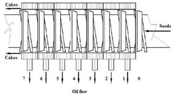
Fig. 3. – Schematic of screw press FL 200 (KABUTEY ET AL., 2010)
