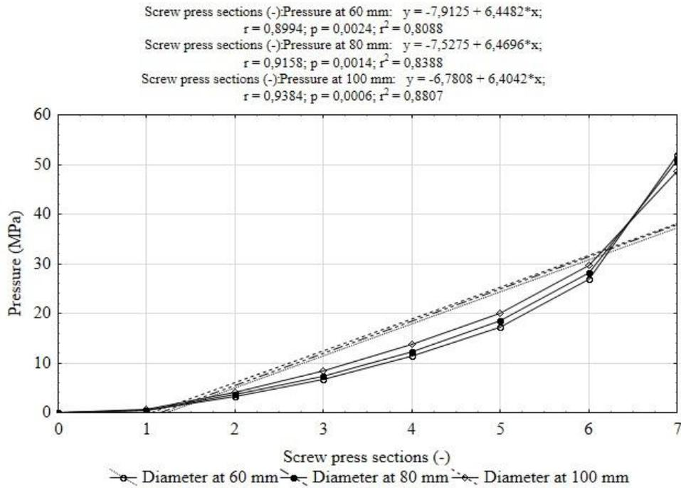
Fig. 5. – Pressure requirement at screw pressing sections of varying vessel diameters applying the tangent model (Eq. 8 and 9)
