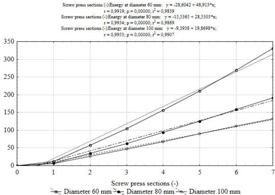
Fig. 6. – Energy requirement at screw pressing sections of varying vessel diameters applying the tangent model (Eq. 10)
