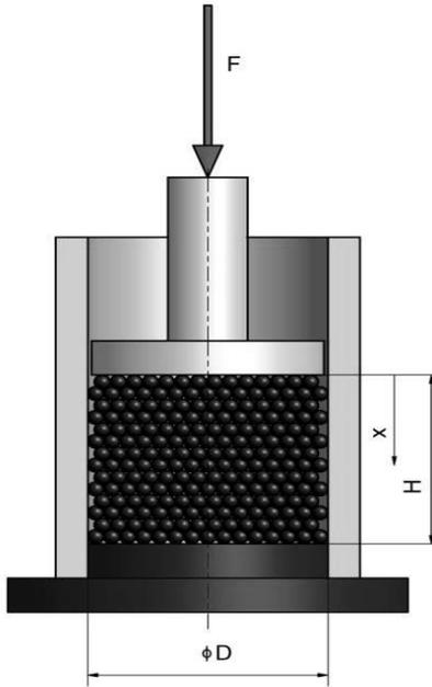
Fig. 2. – Schematic of pressing vessel diameter
