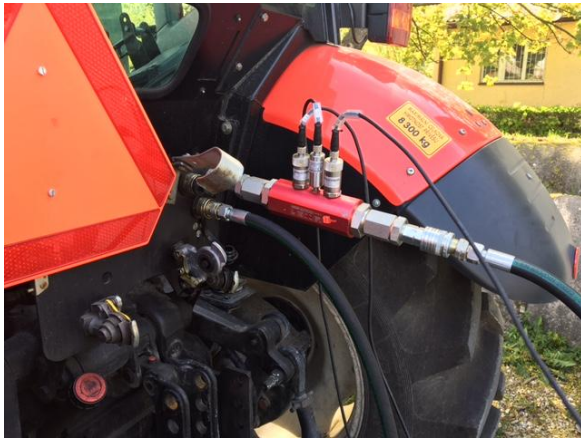
Fig. 2. – Placing of the flow, temperature and pressure sensor on the joint flange HYDAC (Hydac GmbH, Sulzbach/Saar, Germany)
