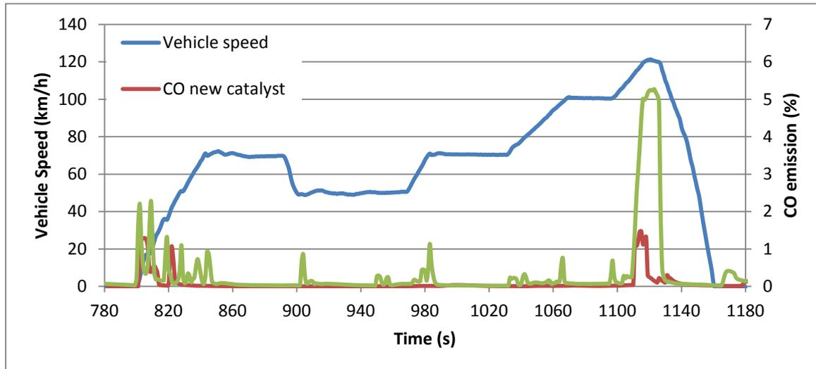
Fig. 2. – Immediate values of CO emissions for both catalysts in the EUDC cycle.
