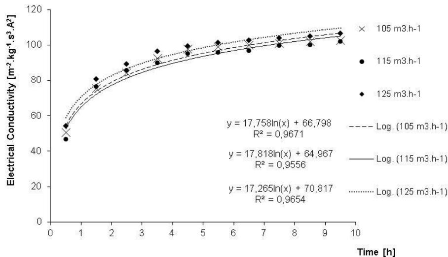
Fig. 3. – Graph of time dependence of electrical conductivity on the air stream of 105, 115 and 125 m<sup>3</sup>.h<sup>-1</sup> respectively
