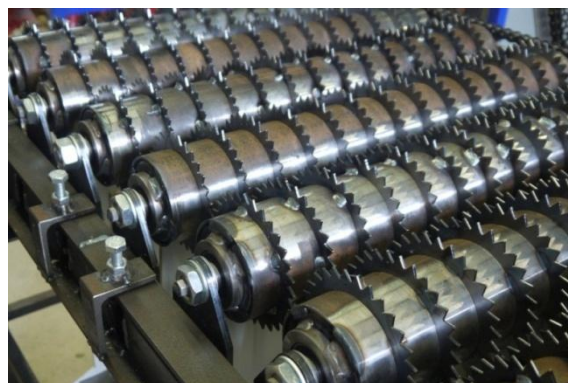
Fig. 2. – Laboratory roller conveyor with rollers fitted with tooth profile welded collars
