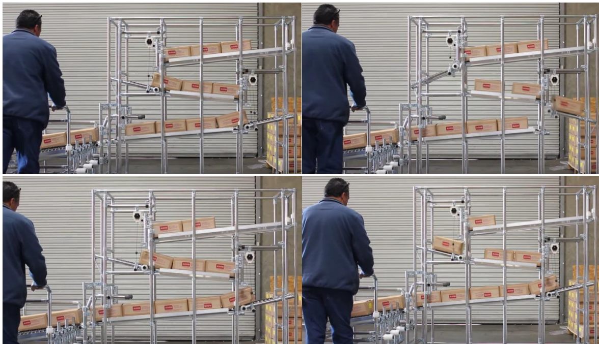
Fig. 2. – Simple karakuri structure for handling operation using gravitation force to provide efficient storage and easy unloading process (AMS, 2014)
