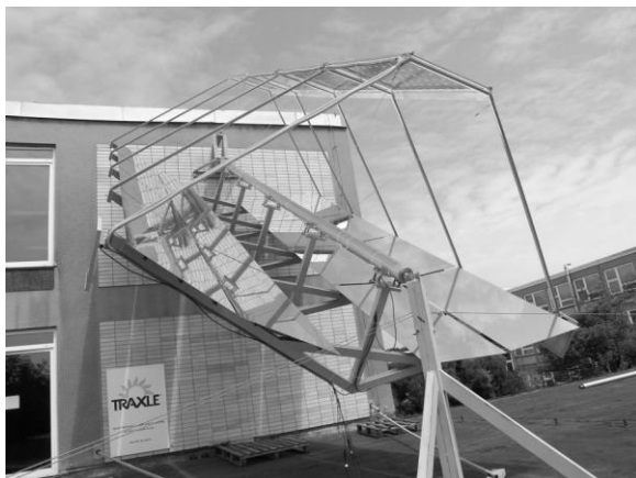
Fig. 5. – Pseudo parabolic concentrator TRAXLE with bifacial PV panels fixed to the building of CULS in Prague
