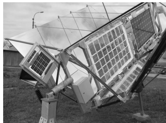
Fig. 8. – Photograph of the 2 nd variant of the tracking pseudo parabolic concentrator with bifacial PV panels in Ryazan
