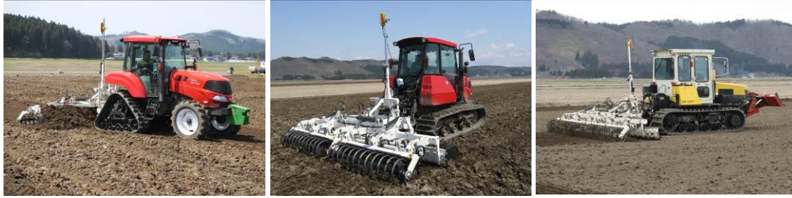
Fig. 1. – Test tractors (Left: Semi-crawler Tractor (EG105), Center: Full-crawler Tractor A (CT1010), Right: Full-crawler Tractor B (MK-140))
