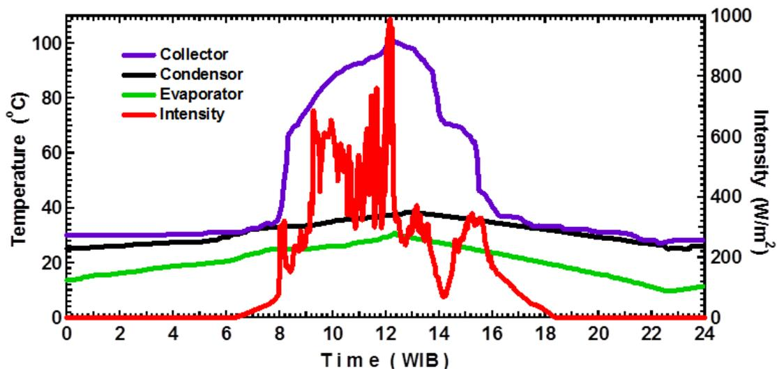
Fig. 7. – The effect of intensity of solar radiation on the component temperature
