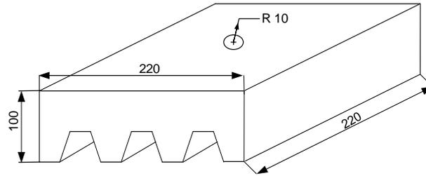
Fig. 3. – Sketch of the evaporator (mm)
