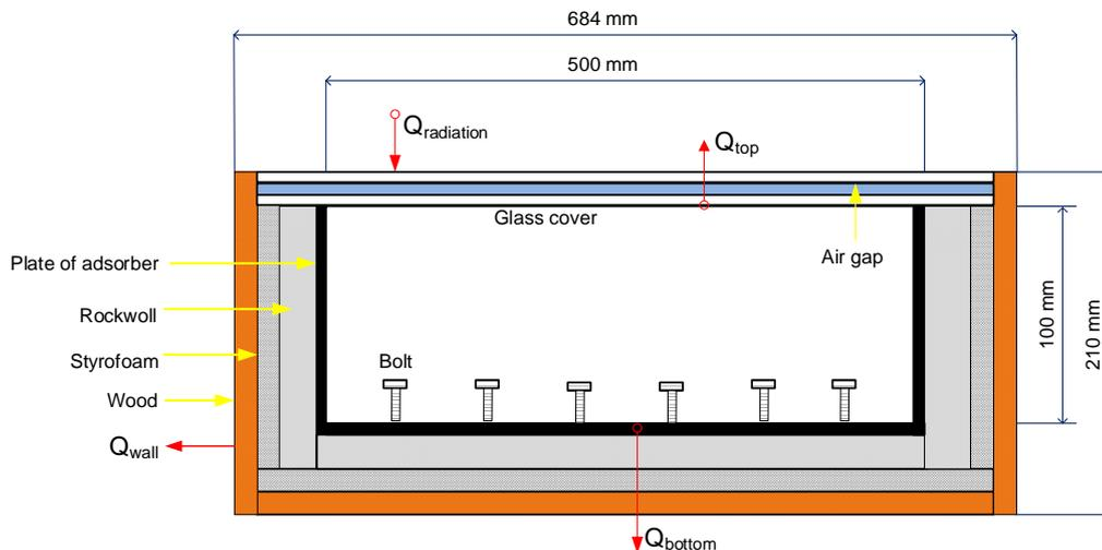
Fig. 2. – The cross section of collector
