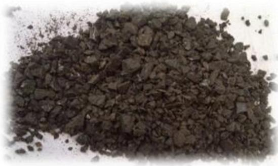
Fig. 1. – Granular activated carbon of Indonesia
