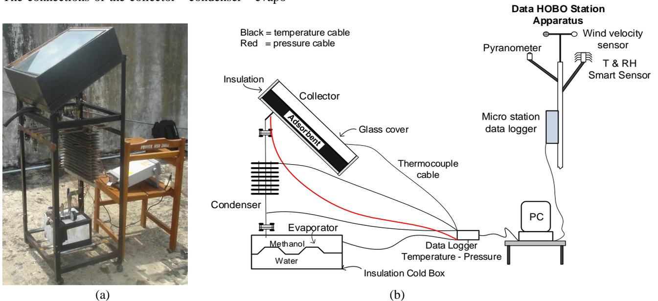
Fig. 4. – (a) Photograph of refrigerator; (b) schematic of refrigerator with measurement systems
