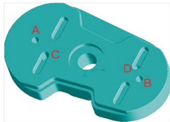
Fig. 3. – Placement of the sensors
