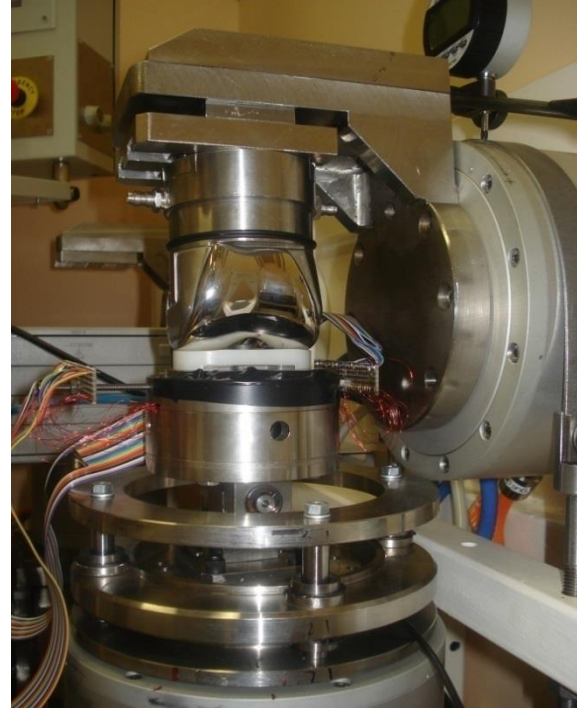
Fig. 5. – Knee movement simulator and artificial joint
