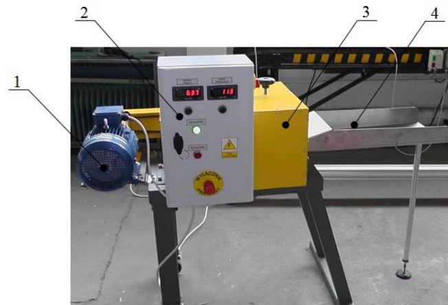
Fig. 10. – Test bed for surveys of the process of cutting with the drum cutting assembly – front view (own study): 1- electric motor with belt transmission, 2 - feed-control system, 3 - feeding-squeezing rollers, 4 - charging gutter
